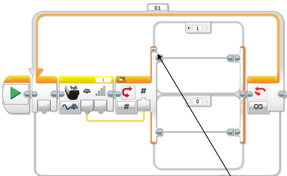
Now we can use a new feature of the EV3 software, Click on the + symbol on the switch. Repeat this 8 times.
