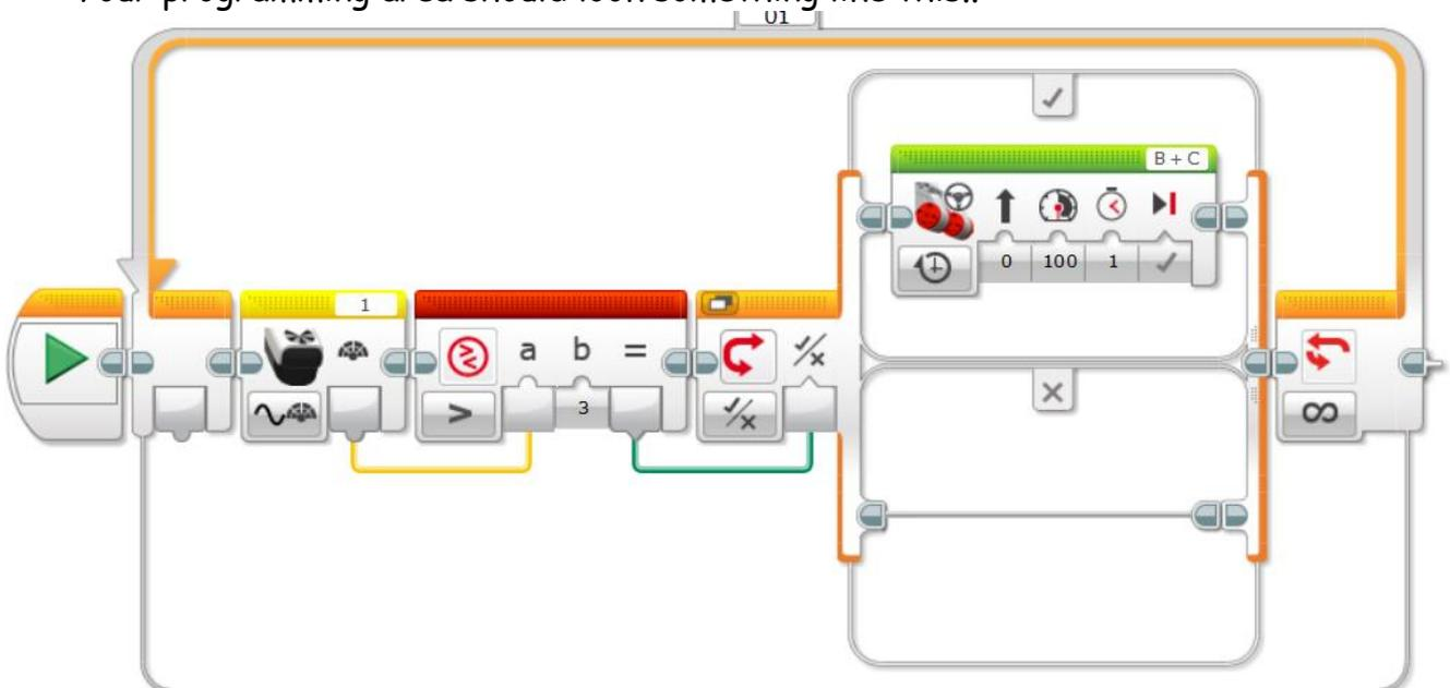
The robot will do nothing until the IRV2 gets a reading greater than 3. Then it will take the top path (True) of the switch and move forwards
