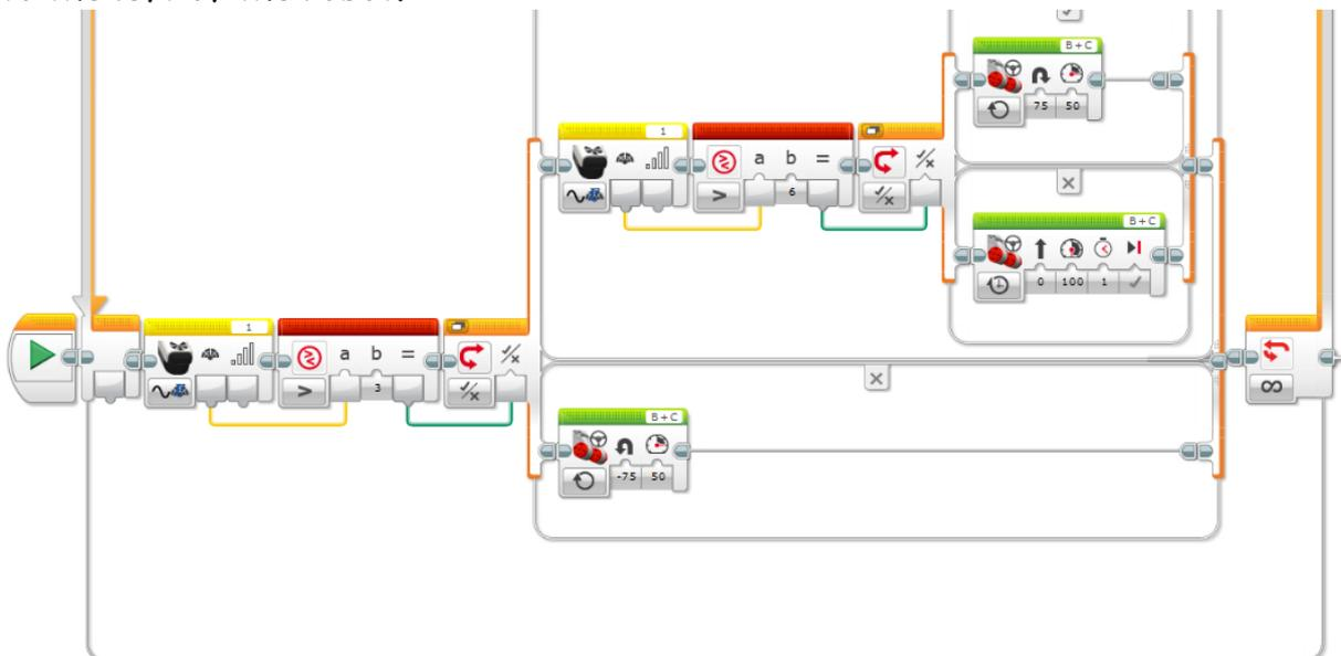
The middle branch is for sensor reading 4,5 and 6 meaning the ball is straight ahead. The top branch is for readings 7,8 and 9, meaning the ball is to the right of the robot.
