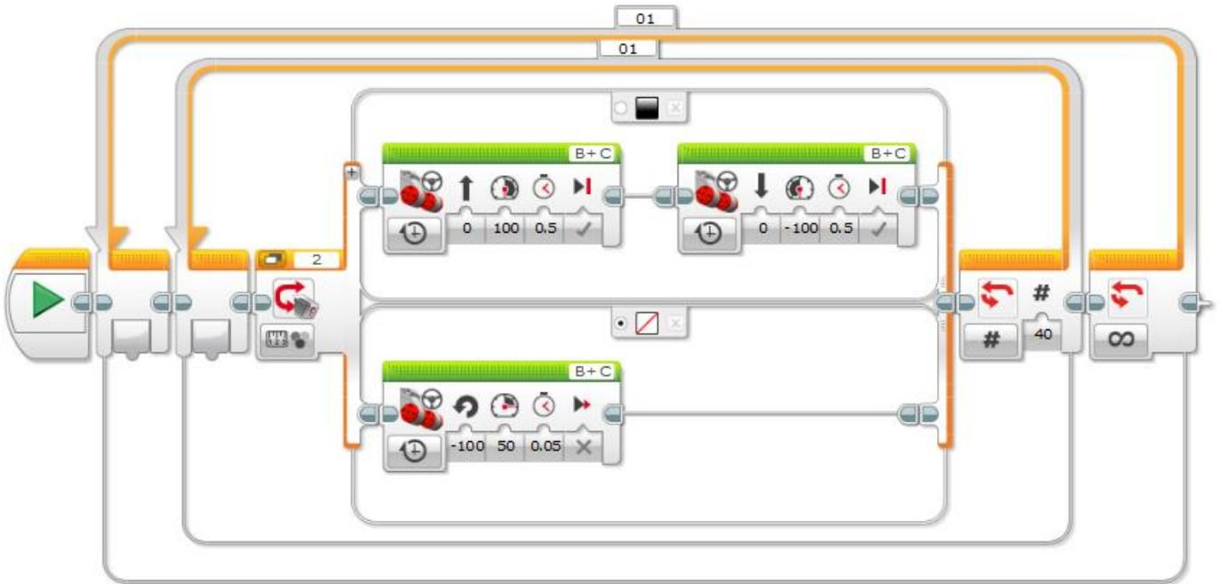
Test the program. The robot will scan to the left and attack the ball when it is close.
