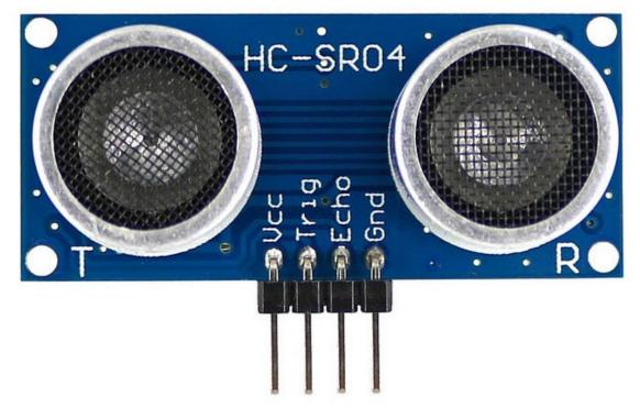
Module size and layout varies between brands. Take measurements off sensor being used.
