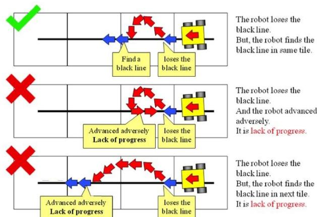
6.4.1.8 The robot fails to reacquire the line before exiting the tile.
